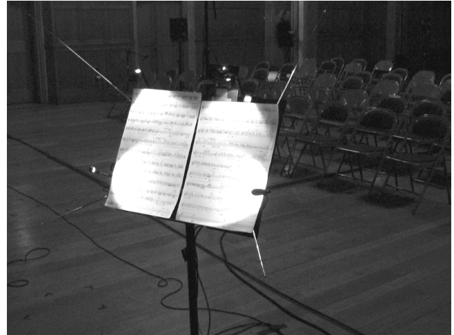
Figure 2: The prototype MMMS with e-field sensor antennas mounted at the corners of the stand.
