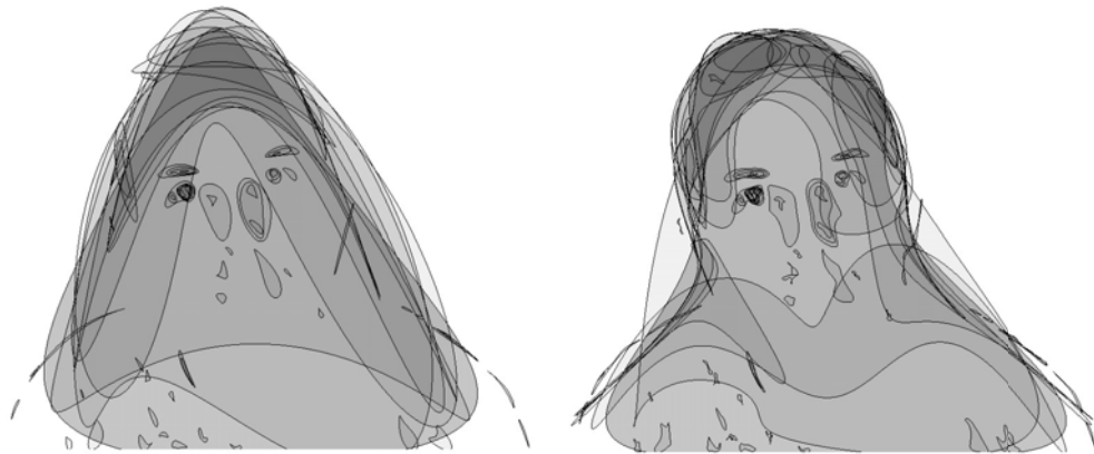
Figure 3.2: Recreating the cumulative connected regions of the input with only three Fourier descriptors (left) and 5 Fourier descriptors (right).
