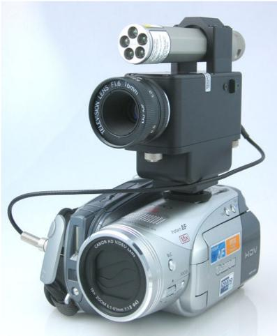
Figure 21. Second generation UVCorder system
