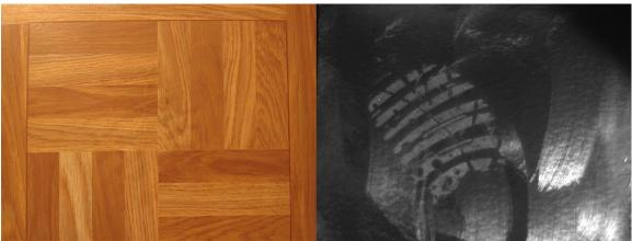
Figure 18. Athletic shoe impression on freshly waxed floor. Left – color, right – near-UV
