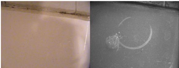
Figure 14. Hair dye ring mark and candle wax trace on bathtub rim. Left – color, right – near-UV
