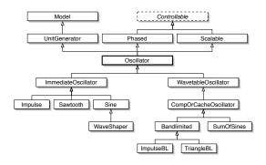
Figure 1: The (partial) class hierarchy of CSL Oscillator UnitGenerators showing multiple inheritance from UnitGenerator, Phased, and Scalable (the last 2 of which are both subclasses of Controllable). The concrete subclasses each implement (at least) a constructor and a *nextBuffer* method.
