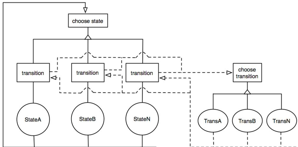
**Figure 20. Embedded Transition State pattern**
