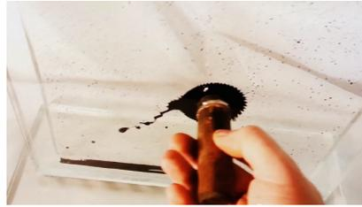
**Figure 2.2:** *Prototype Glass Ferrofluid Display* Casey Hughes (2013) [8]
