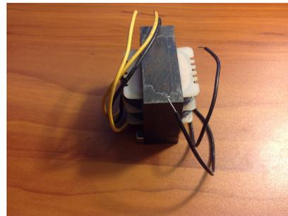
**Figure 3.11:** Transformer as purchased, before being re-built as electromagnet.
