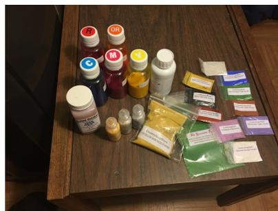
**Figure 3.4:** Coloring agents used to mix with ferrofluid: liquid dyes, several colors of iron oxide powder, others.
