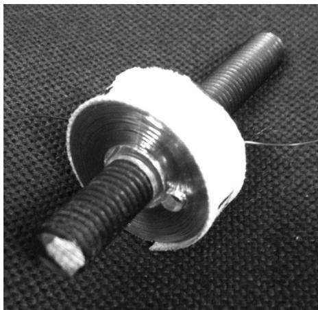
Figure 4.1: Electromagnet coil on steel bolt.
