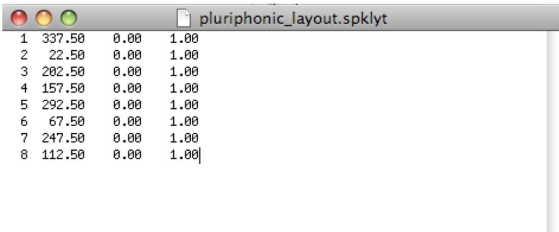
The simple column based text format of .spklyt files allows for easy tweaking in a text editor outside of SES, or one may paste the columns into a spreadsheet application like Excel for more advanced editing. The example in Figure 9 corresponds to the layout in Figure 8. The first column is the speaker number followed by the azimuth, elevation, and distance for each speaker.
