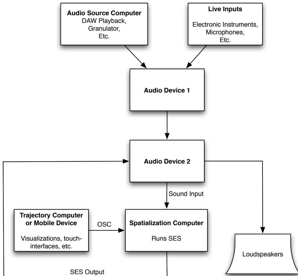
**Figure 2. Distributed Processing with SES Over Two Computers**
