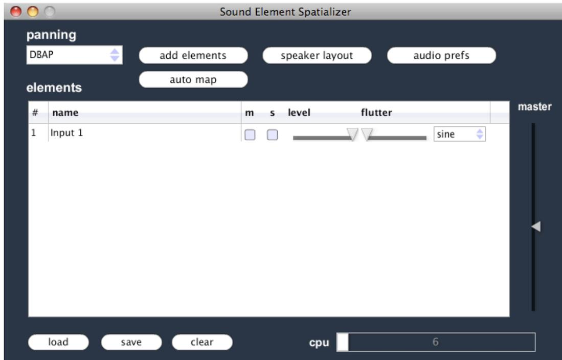
By default the first input from the audio device is mapped to a single element. To add more elements, the user can click the “add elements” button on the main window, which reveals the window shown in Figure 11. Alternatively, the user may select the “auto map” button, which will automatically map each input channel of the audio device to a separate element.
