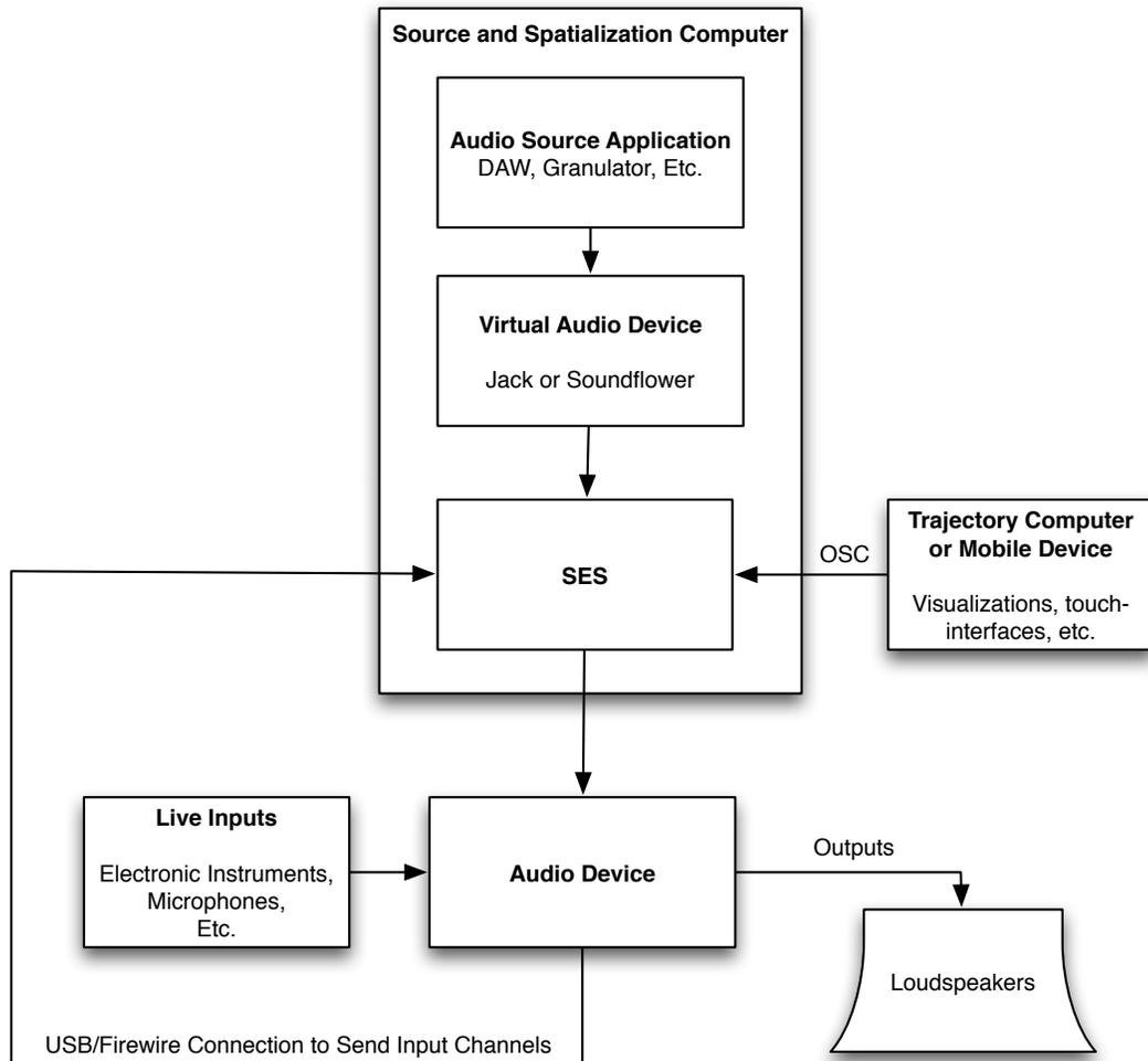
Using a virtual audio device such as Jack [27] or Soundflower [28], one may realize a complete spatialization system with SES on a single computer. The user routes output from the sound generating application to SES through the virtual audio device and configures the OSC trajectory controller to use the network address of localhost (127.0.0.1).
