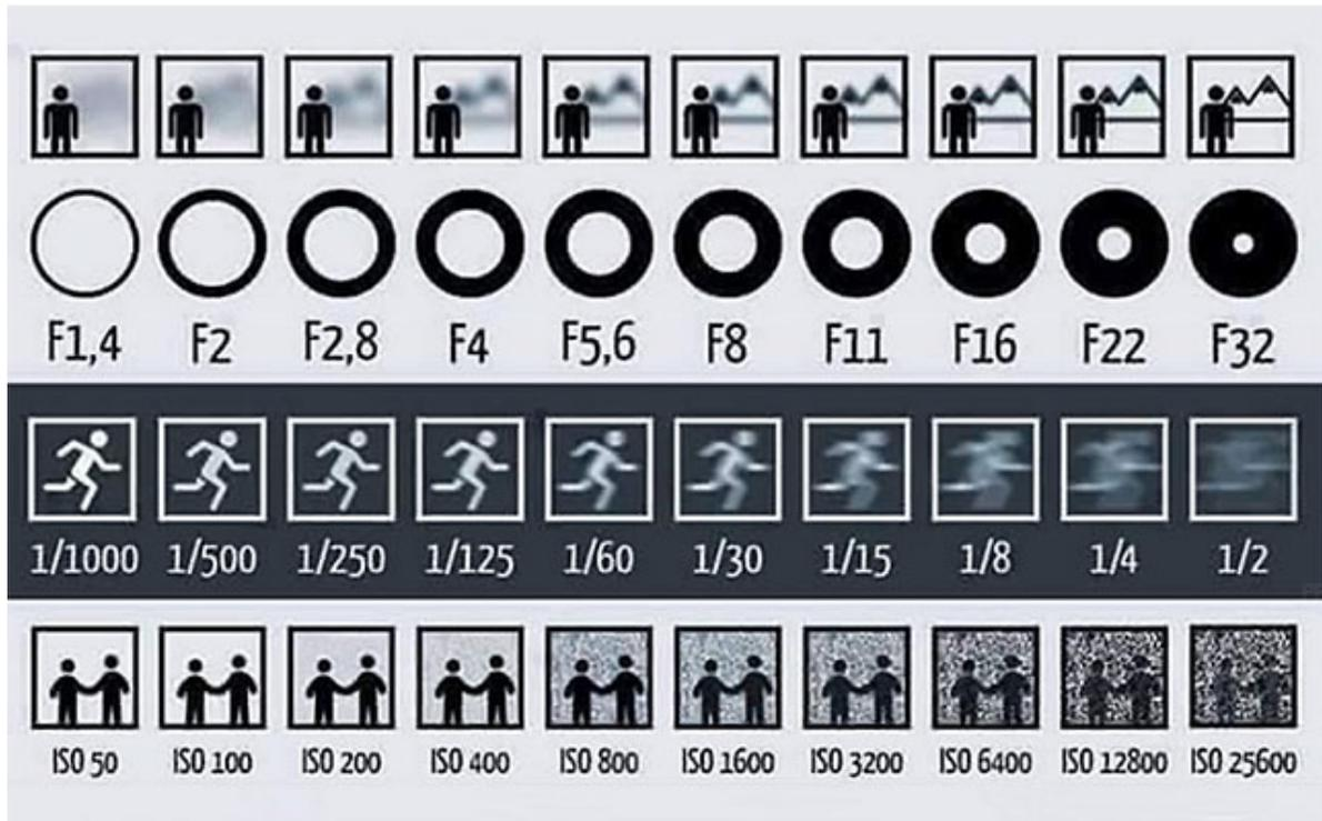
**Figure 23. Visual effect of camera parameters on the image (Petapixel)**
