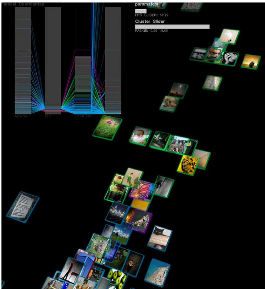
**Figure 1. Image organization in 3D space with K-means clustering. The border color around the image represents the cluster it belongs to.**
