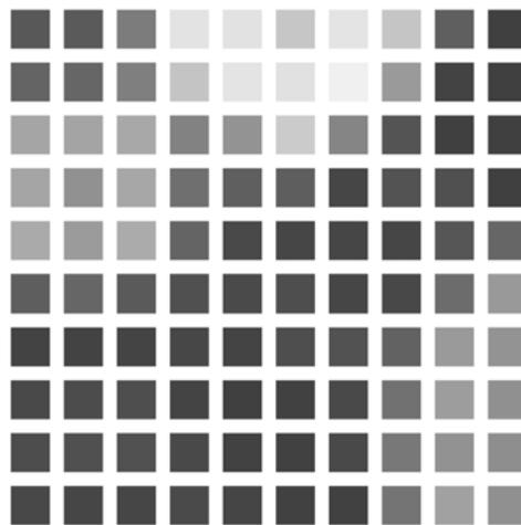
**Figure 11. U-Matrix: the color of the node represents the mean Euclidian distance between its weight and the weight of its 4 neighbors**
