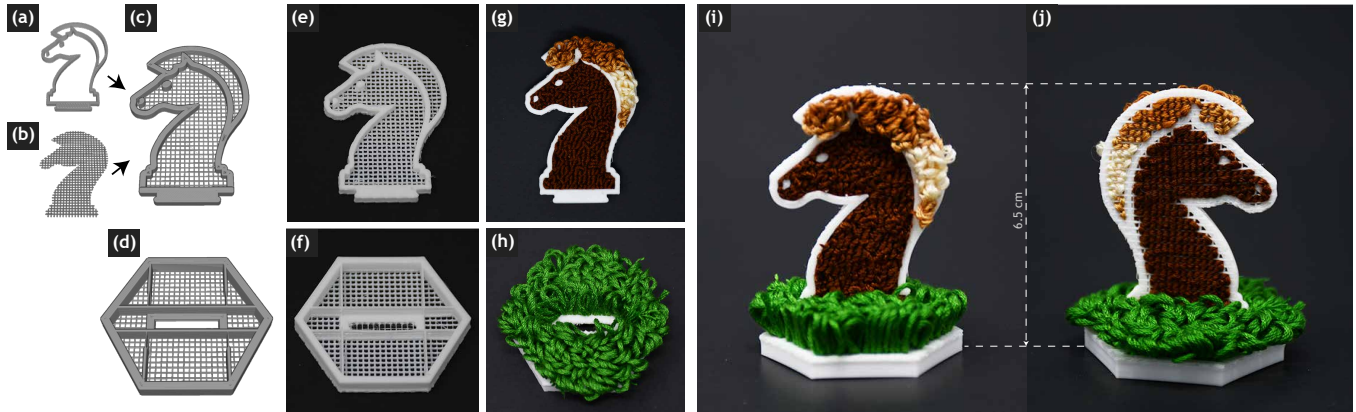
Figure 11: PunchPrint design workflow enables integration of our fabric method and complex geometry sliced with commercial slicers in the same print. It also creates an opportunity in assembling punched pieces together using press fit methods: (a) Surrounding geometry sliced with Cura; (b) our fabric generated in Grasshopper; (c) inserting the fabric GCode into sliced GCode results in a unified form; (d) the same procedure as in (a)-(b) repeated for the base of knight; (e) fabricated and (g) punched knight piece; (f) fabricated and (h) punched base piece; (i) the looped and (j) flat sides of the final artifact (6.5 cm).
