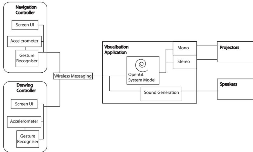
Figure 4: Functional Diagram of Gesture
