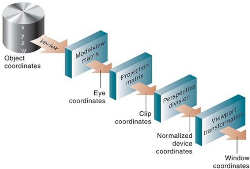
Figure 16: The OpenGL Vertex Transformation [43]
