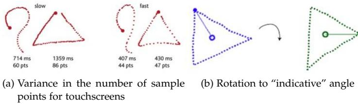
Figure 7: \$1 Recognizer - Key steps [51]
