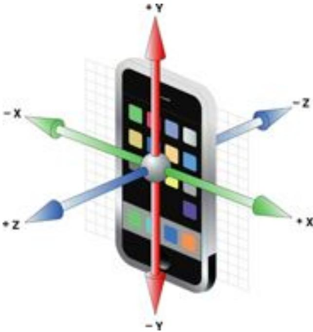
Figure 8: The iPhone as an Accelerometer[5]
