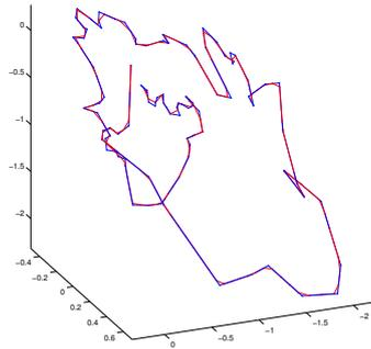
Figure 13: Raw Accelerometer data for a Circle Gesture (Also shown is resampled data for first step of gesture recognition)
