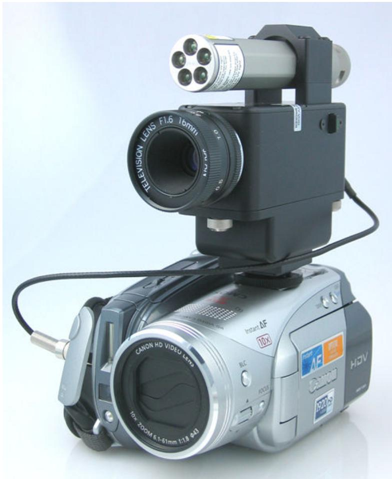
**Figure 21. Second generation UVCorder system**
