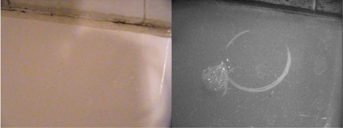
**Figure 14. Hair dye ring mark and candle wax trace on bathtub rim. Left – color, right – near-UV**
