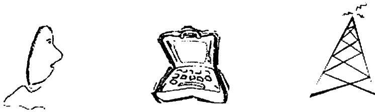
Figure 5.17 In the third architecture, devices talk to local base stations (like computers or repeaters) within rooms. Signals have to travel about 20 meters.
