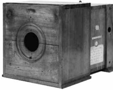
The world's first camera, known as the "chambre de la découverte" (the chamber of discovery), made by Nicéphore Niépce before 1826. Sliding box camera. 30.5 x 31.5 x 25 cm.
