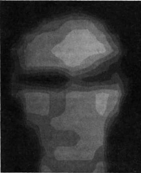
of 16 levels of gray. Not all the 256 squares are required to represent the face. The contoured representation at right was produced by filtering the block portrait to remove high frequencies.
