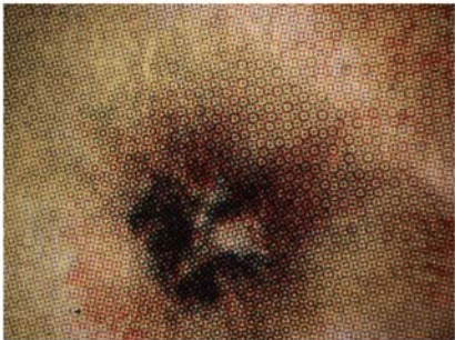
Figure 21a Microscopic detail of fig. 20, recorded at 10× magnification, showing superposition of all four color print layers.
