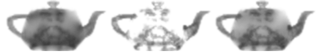
Figure 6: Left: Solution \omega^{i-1} after one optimization pass. Middle: The reinforcement structure V from \omega^{i-1} . Right: Extension field \beta of V .
